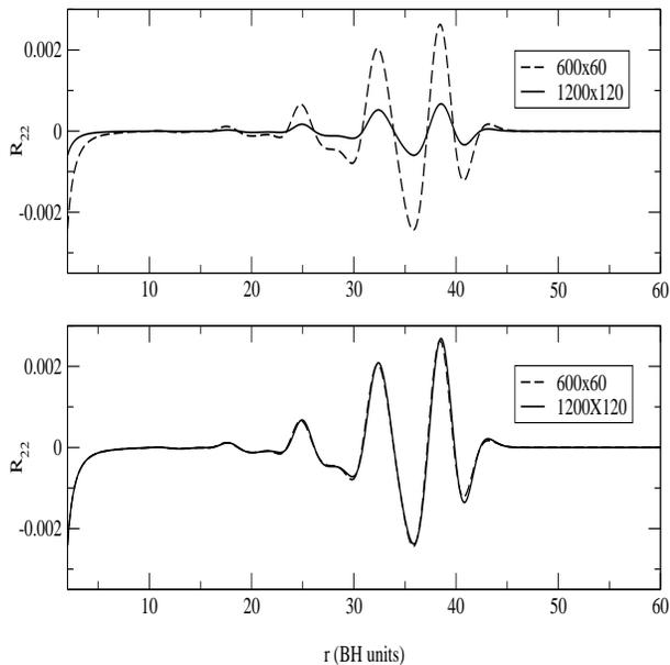
FIG. 2: Convergence test for the  $R_{22}$  component of the Ricci tensor. The top panel shows this component for two different resolutions for a radial slice on the equatorial plane. As expected the value is converging to zero. In the bottom panel we have tested the second order power law of convergence by multiplying the 1200x120 output by a factor of four. The two curves now overlap perfectly, thus proving second order convergence.
