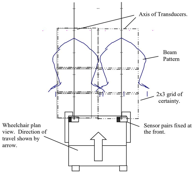
**Fig. 3.** Representation for a two-sensor array.
