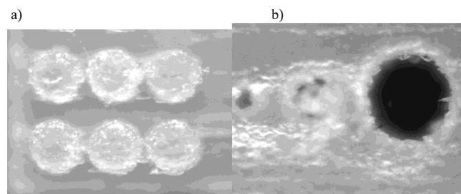
Fig. 6. a) Cylinders of 0.5mm; (b) Hole of 1mm.
