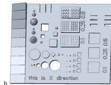
Fig. 3. a) BMP with small geometrical features (overall size: 75mm x 54mm x 15mm); b) BMP with mezzo features (overall size: 27mm x 22mm x 3mm).
