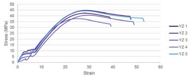
Fig. 10. Tensile stress-strain diagram in Y-Z plane.
