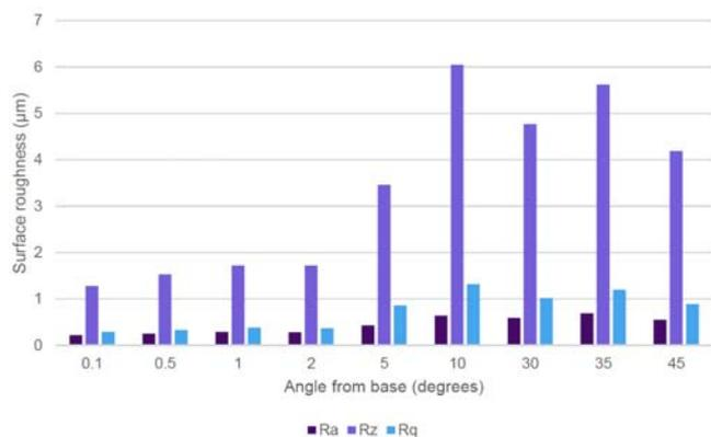
Fig. 4. Surface roughness against the surface angle.
