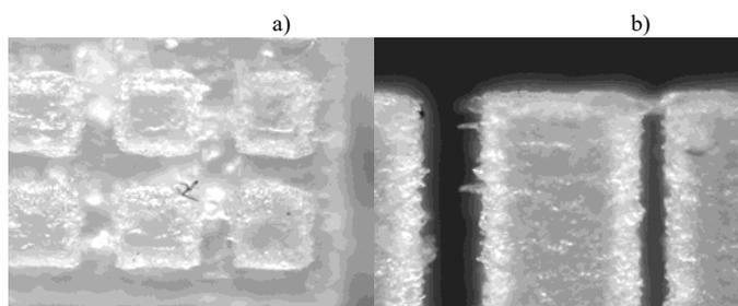
Fig. 5. a) Cuboids of 0.5mm; b) Slots of 0.5mm and 0.25mm.
