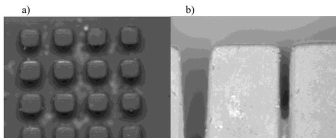
Fig. 13. a) Cuboids of 0.25mm; b) Slots of 0.5mm and 0.25mm.
