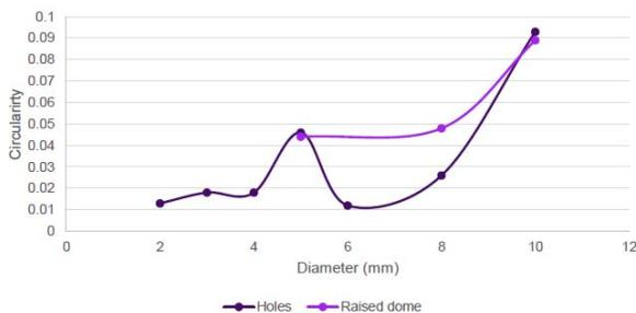
Fig. 8. Circularity (mm) of the holes and domes.
