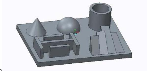
Fig. 12. BMP for geometrical accuracy: a) positional accuracy; b) geometrical shapes and surface roughness.
