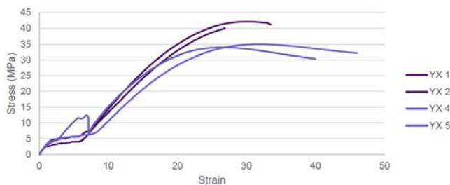
Fig. 9. Tensile stress-strain diagram in X-Y plane.
