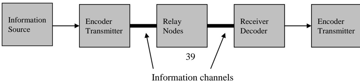
Fig 71.9: Components of a Fibre Optic Communication System
