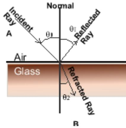
Fig 71.3 Reflection and Refraction
