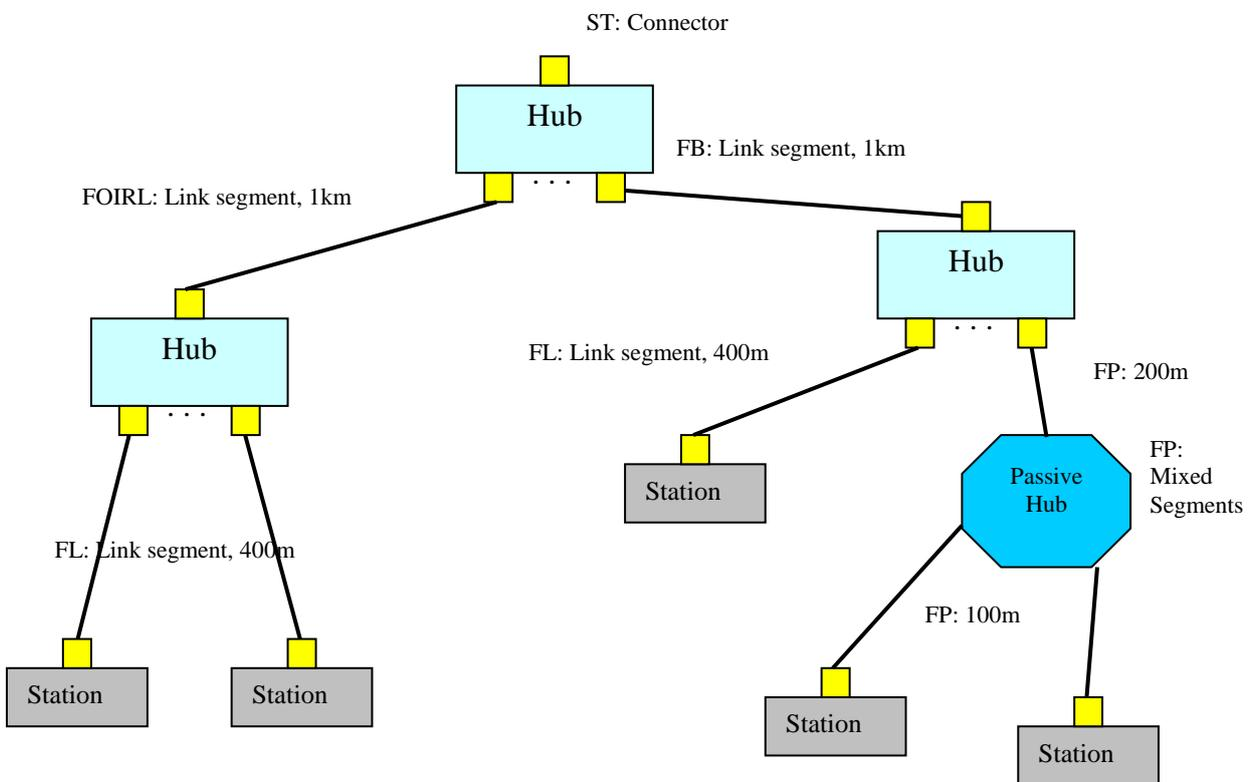
Fig 71.13: Mixed Optical LAN with 10BASE-F connections.
