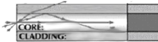
Fig 71.6 Total internal reflection in multimode step-index fibre
