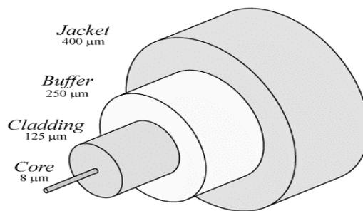
Fig 71.4: The structure of a fibre optic cable
