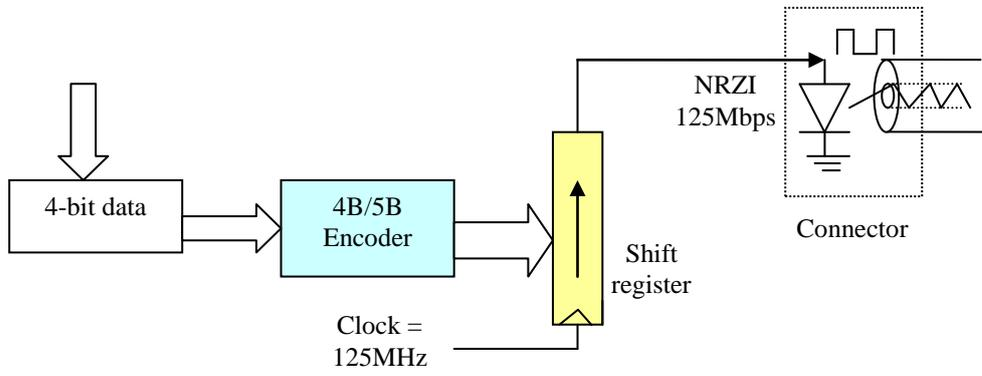
Fig 71.14: Encoding sequence for 100BASE-FX, which adopts the 4B/5B-encoding scheme
