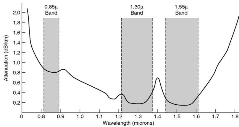
Fig 71.8: Attenuation (dB/Km) in a silica-based optical fibre
