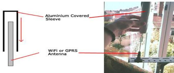
Figure 6 – Simulating Roaming with antenna sleeve
