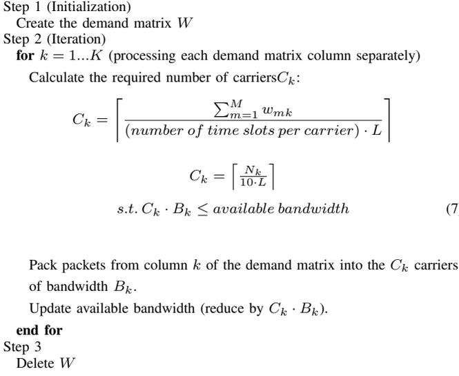
Figure 1. Allocation algorithm
