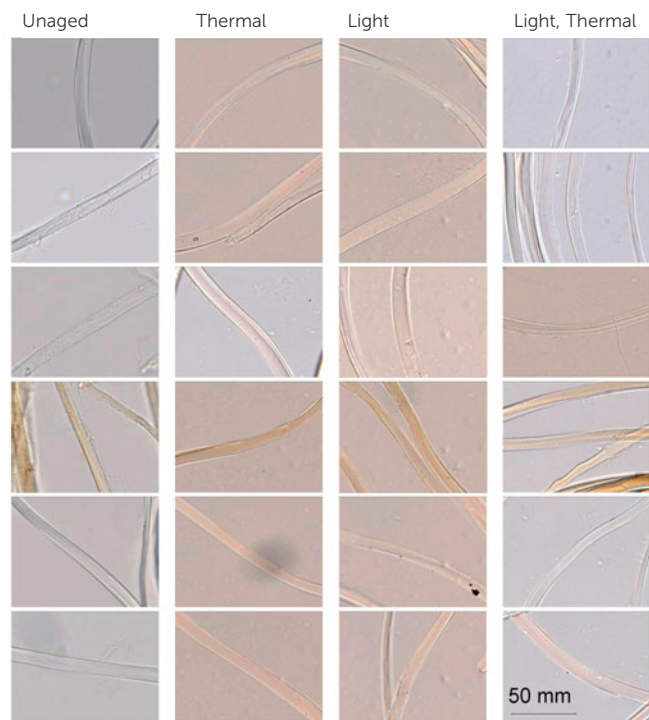
Figure 1: Typical light micrographs of weighted and aged silk fibres.
