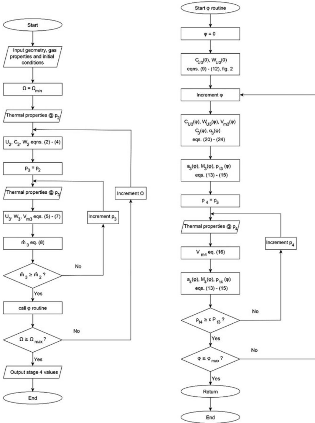
**FIGURE 4** Flow chart for the analytical model
