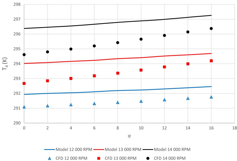
**FIGURE 9** Comparison of the diffuser outlet temperature computed by the 1D analytical model the 3D CFX simulation for increasing vane angles  $\phi$
