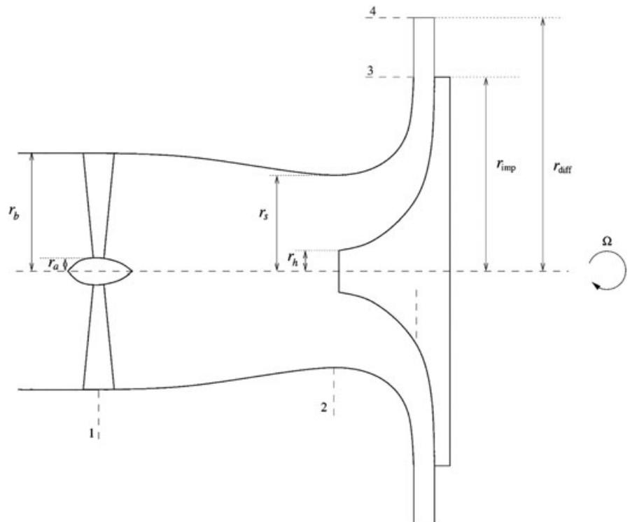
**FIGURE 1** Compressor geometry and the 4 stages considered in the 1D model
