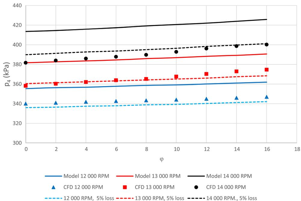
**FIGURE 10** Diffuser outlet pressure from the 1D analytical model with a 5% diffuser loss
