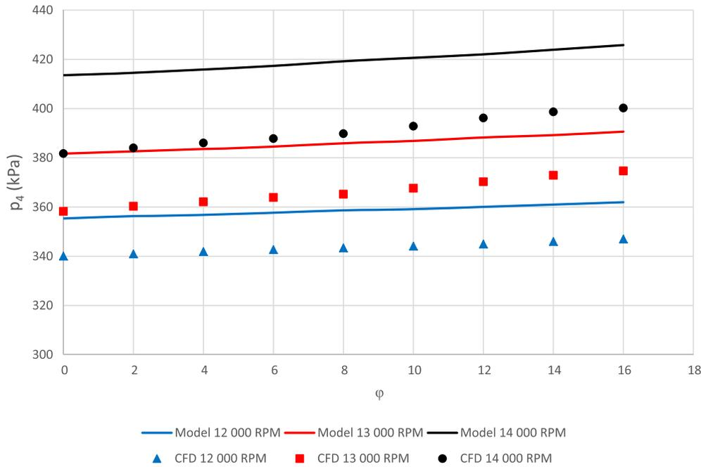
**FIGURE 8** Comparison of the diffuser outlet pressure computed by the 1D analytical model the 3D CFX simulation for increasing vane angles  $\phi$
