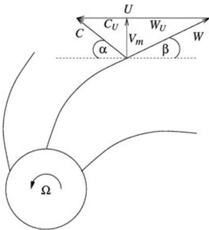
FIGURE 2 Details of the velocities at the tip of the impeller
