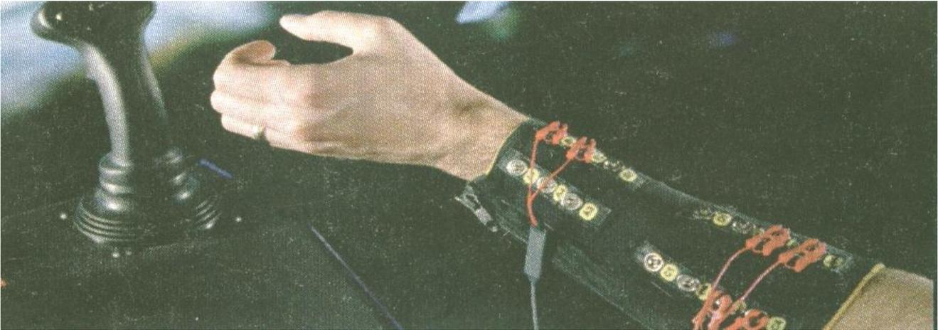
Figure 4: Arm Glove to sense nerve voltages
