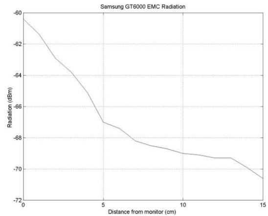
Figure 6 : EMC Radiation from a Samsung monitor.
