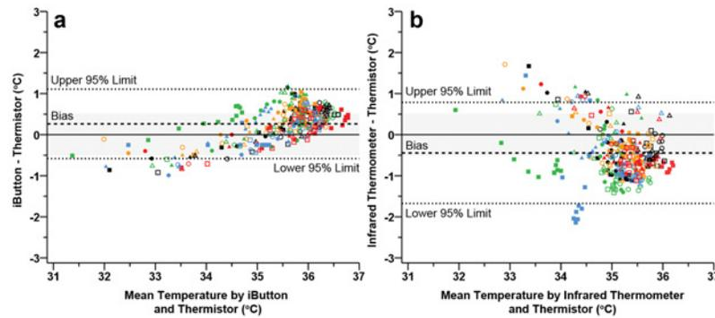
**Fig 3. Bland—Altman plots during exercise in the heat illustrating the mean bias (dashed line) and 95% limits of agreement (mean difference  $\pm 1.96 \cdot$  modified standard deviation: dotted lines) for thermistors vs iButtons (a), thermistors vs infrared thermometer (b). Each participant is represented by a unique colour or shape ( $n = 30$ ). Grey band indicates the practically meaningful, a priori acceptable mean bias ( $\pm 0.5^\circ\text{C}$ ).**
