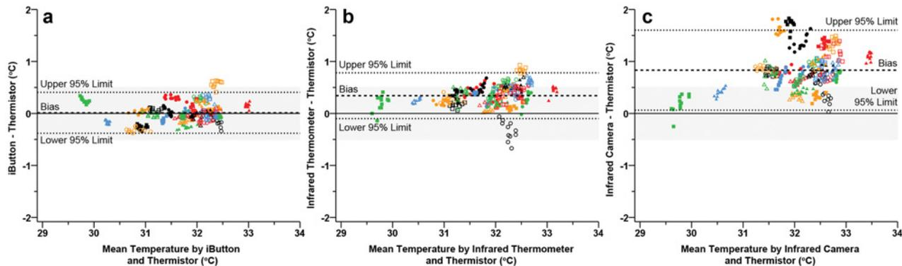
**Fig 2. Bland—Altman plots during rest illustrating the mean bias (dashed line) and 95% limits of agreement (mean difference  $\pm$  1.96  $\cdot$  modified standard deviation: dotted lines) for thermistors vs iButtons (a), thermistors vs infrared thermometer (b) thermistors vs infrared camera (c). Each participant is represented by a unique colour or shape ( $n = 30$ ). Grey band indicates the practically meaningful, a priori acceptable mean bias ( $\pm 0.5^\circ\text{C}$ ).**
