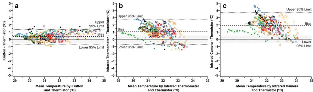
**Fig 4. Bland—Altman plots during recovery illustrating the mean bias (dashed line) and 95% limits of agreement (mean difference  $\pm$  1.96  $\cdot$  modified standard deviation: dotted lines) for thermistors vs iButtons (a), thermistors vs infrared thermometer (b) thermistors vs infrared camera (c). Each participant is represented by a unique colour or shape ( $n = 30$ ). Grey band indicates the practically meaningful, a priori acceptable mean bias ( $\pm 0.5^\circ\text{C}$ ).**
