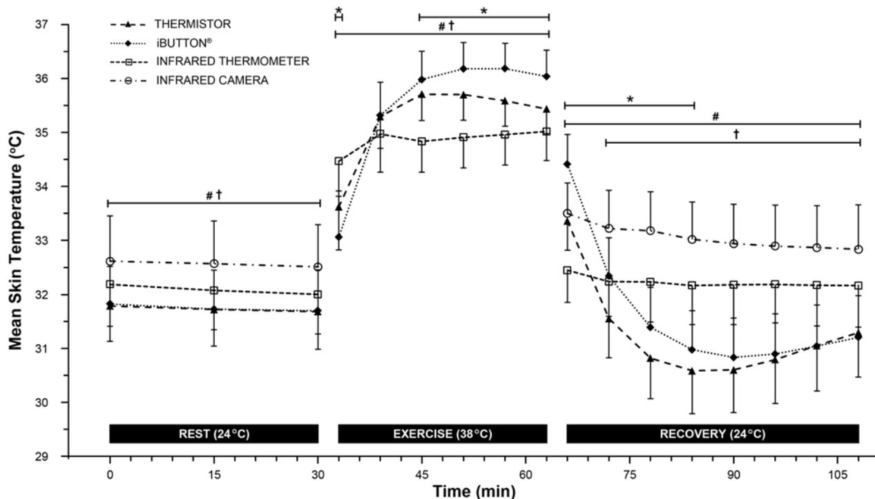
**Fig 1. Mean skin temperature (n = 30) of all tested devices during rest (4 devices), exercise (3 devices) and recovery (4 devices).** Post-hoc analysis displayed as \*Significant differences between iButtons and thermistors ( $p < 0.001$ ); #Significant differences between infrared thermometer and thermistors ( $p < 0.001$ ); †Significant differences between infrared camera and thermistors ( $p < 0.001$ ). Results are presented as the mean  $\pm$  SD.
