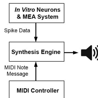
**Figure 1.** The overall architecture of the instrument.
