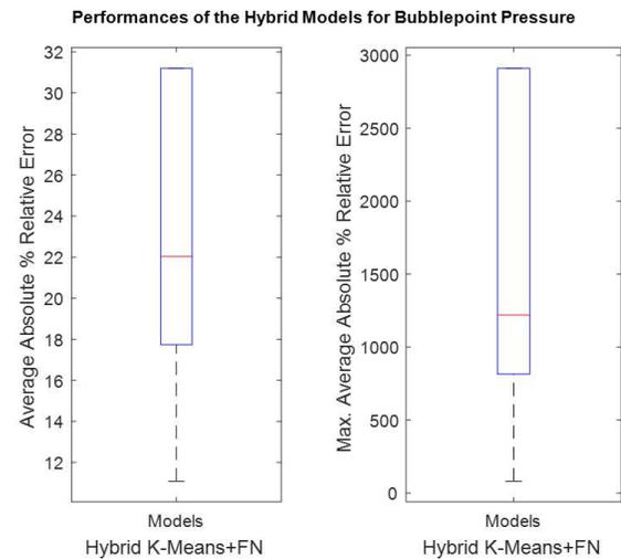
Fig. 5.  $P_b$  Boxplot for K-Means+FN and  $E_a/E_{max}$
